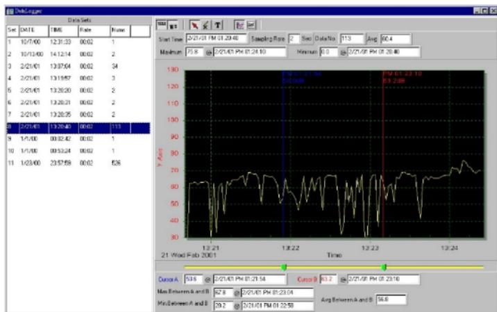
Once the meter is connected to the PC, either select “DataLogger” from the main menu or click on
